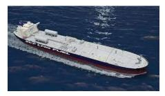
China State Shipbuilding Corporation Limited's (CSSC) first liquefied natural gas dual fuelled very large crude carrier for COSCO Shipping began sea trials recently. The vessel is 332.6 metres long and has a deadweight tonnage of 318,000. The vessel is a dual fuelled VLCC and uses LNG as its main fuel which is further supplemented by fuel oil. The vessel is also equipped with dual-fuel generators and dual-fuel boilers.
