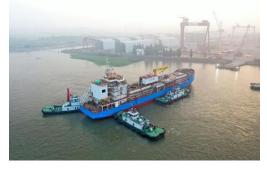
The 7,500 cubic metre liquefied natural gas bunkering vessel (LBV), the "FUELNG BELLINA" was delivered early last week to FueLNG. The vessel is the world's first smart LNG bunkering vessel and was designed by Keppel Offshore & Marine's (Keppel O&M) technology arm, Keppel Marine and Deepwater Technology. It was built in Keppel O&M's Nantong shipyard. FueLNG is a joint venture between Keppel O&M and Shell Eastern Petroleum (Pte) Ltd.
