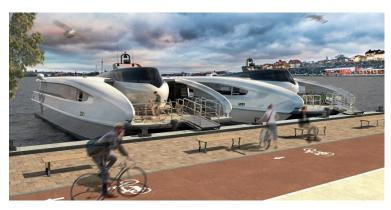
Green City Ferries ("GCF") has launched the BELUGA 24, a revolutionary zero emission passenger ferry which is set to service the Swedish city from 2023. aerodynamic, twin-hulled catamaran will have a capacity of 150 passengers and 30 bicycles.
